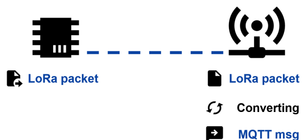
Figure 5.20: Converting between a LoRa packet to MQTT
