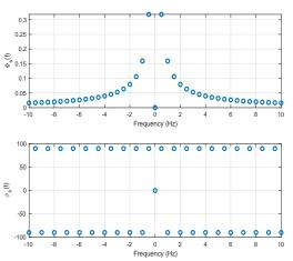
Power spectral density (top) and phase spectrum (bottom)
