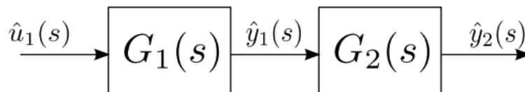
$$\begin{aligned}\hat{y}_2(s) &= G_2(s)\hat{y}_1(s) \\ &= G_2(s)G_1(s)\hat{u}_1(s)\end{aligned}$$
