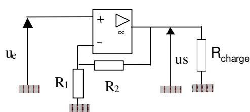
$$u_s = \frac{R_{charge}}{R_{charge} + Z_s} T u_e$$
