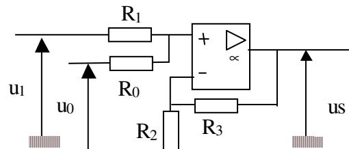
$$u_s = \left( 1 + \frac{R_3}{R_2} \right) \left[ \frac{R_1}{R_1 + R_0} u_0 + \frac{R_0}{R_1 + R_0} u_1 \right]$$
